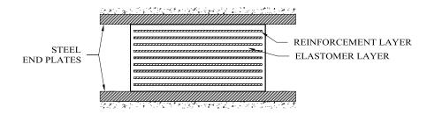
*Figure 1: Typical Elastomeric Bearing (note: the steel end plates are not necessarily required)*
