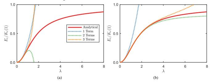
Figure 4: Comparison of the analytical solution for  $E_c$  to the truncated Taylor series expansion of the (a) original expression and (b) inverted expression.
