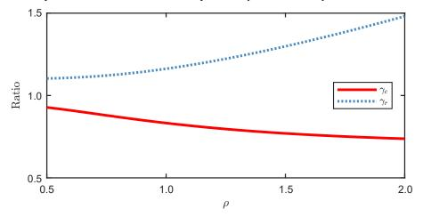
Figure 3: Ratio of the shear strain determined from the CHBDC to the analytical solution assuming an incompressible elastomer and inextensible reinforcement.
