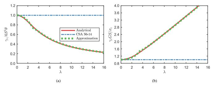
Figure 6: Comparison of the analytical solution to the proposed approximation and the CHBDC equation for (a)  $\gamma_r$  and (b)  $\gamma_c$ of a circular pad
